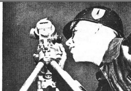
Candidate Wayne Smoot of Newcastle, Calif., sights through the eyepiece of a theodolite (a survey instrument)
